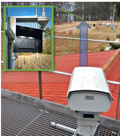
\text{NH}_3 Open Path Compact set up at the Federal Environmental Agency station Neuglobsow, Germany (left). Example data time series (right).
