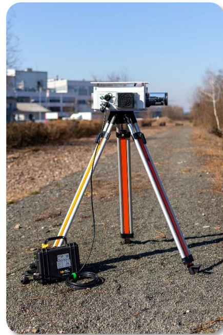
SkySpec Mini in the field with tripod and LiPo battery pack (available accessories)
