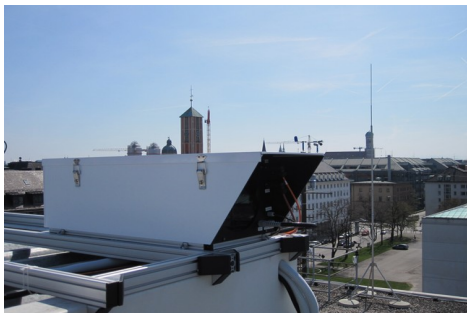
Open Path telescope unit, mounted on a roof top (telescopes are customised and may look different).
