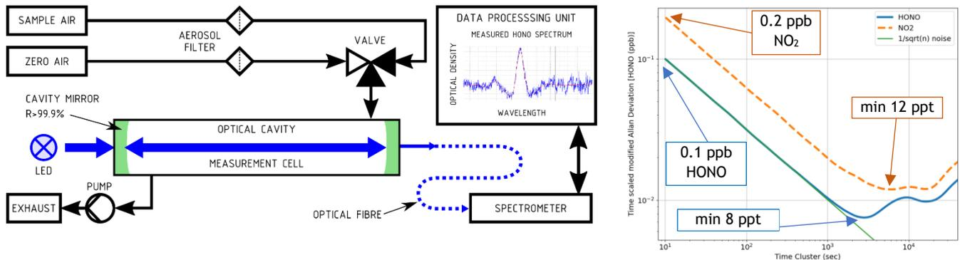
Flow scheme and Measurement Principle of the ICAD HONO / NO<sub>2</sub> measurement system.
