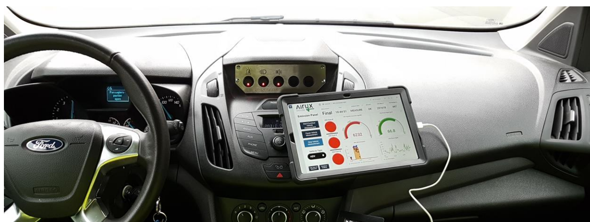
Figure 7: Display installation in the cockpit. A tablet is used to display the real time data and is connected via WiFi to the ICAD instrument. It allows operation and visualisation.
