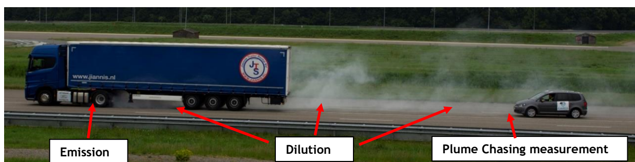
Figure 8: Illustration of plume chasing measurement configuration. The emitted exhaust gases are diluted. The plume chasing vehicle measures the gases in the diluted plume. Exhaust gases visualised in this picture with white smoke.
