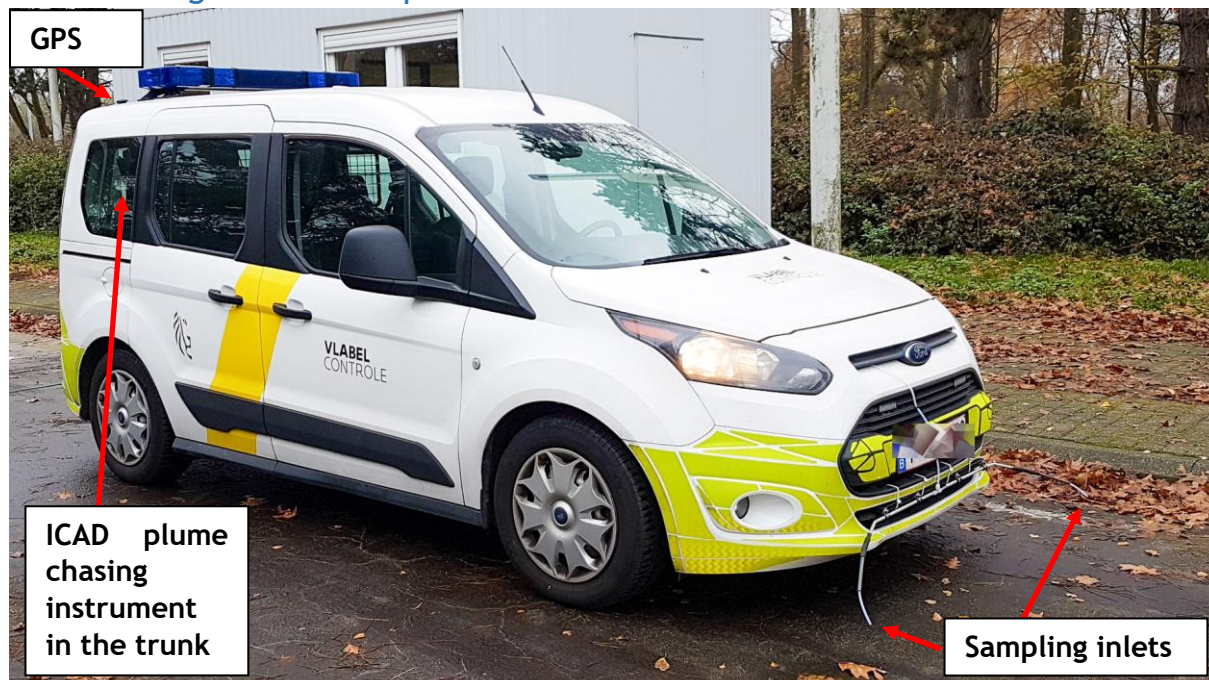
Figure 4: Plume chasing installation on the Vlabel Controle vehicle (outside view). Two sampling inlets are combined to one sampling hose to the ICAD plume chasing instrument in the trunk.
