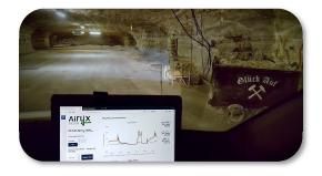
The high mobility, rugged design, and low maintenance effort make ICAD instrument the ideal instrumentation for reliable monitoring  $NO_x$  levels in workplace environments such as mines, constructions site or industrial production places. Further, ICAD instruments can be applied to measure and monitor the  $NO_x$  emissions of industrial machines. Multiple data interfaces enable optional integration of ICAD instruments with industrial processes.
