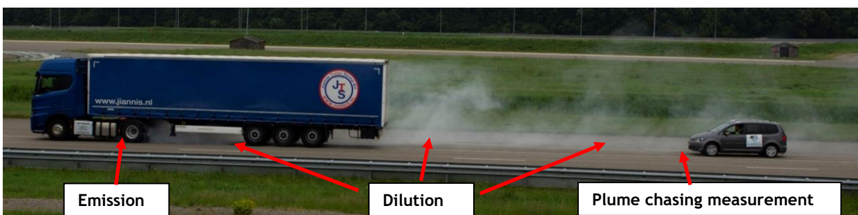
Figure 10: Illustration of plume chasing measurement configuration. The emitted exhaust gases are diluted. The plume chasing vehicle measures the gases in the diluted plume. Exhaust gases visualised in this picture with white smoke.
