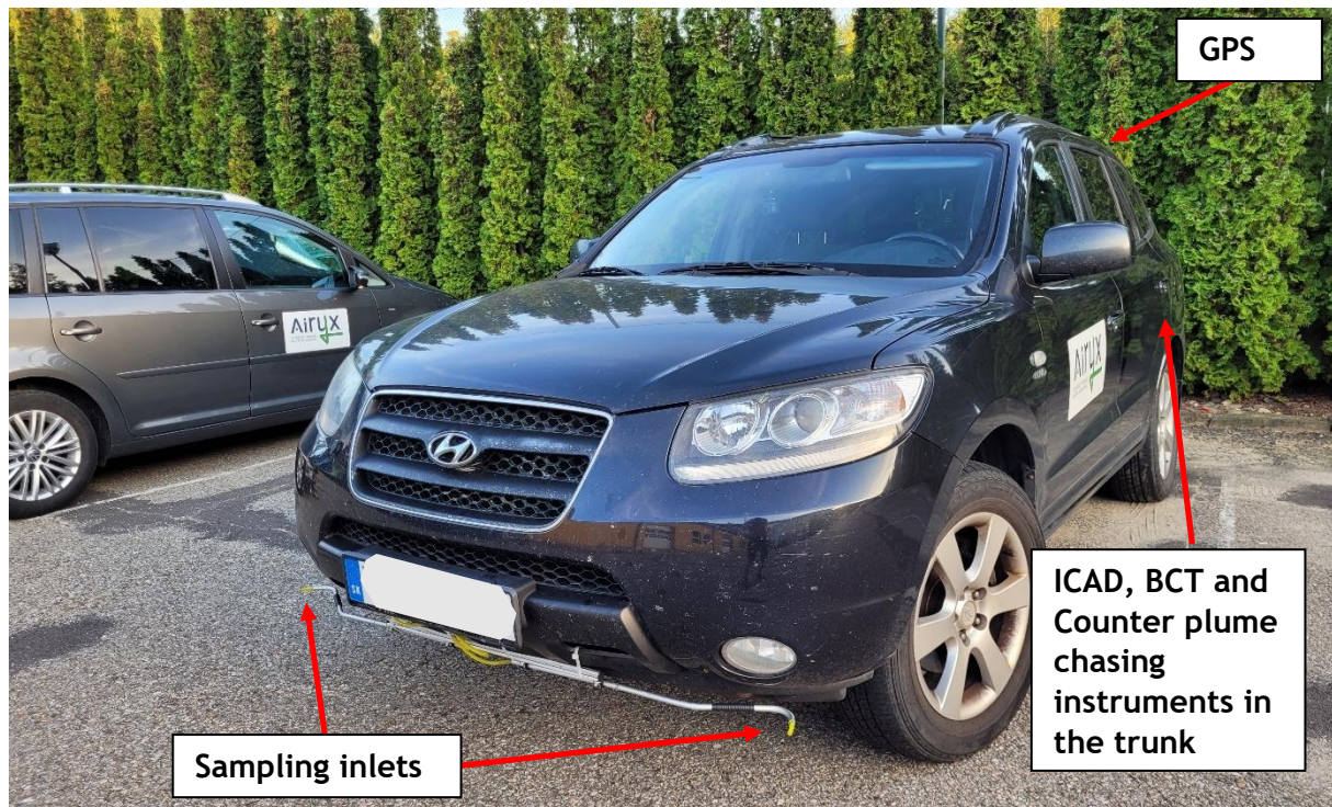
Figure 5: Plume chasing installation on ChasingVeh2 (outside view). The measurement probe system features two sampling inlets which are combined to one sampling hose to the ICAD plume chasing instrument, Counter, and BCT in the trunk.
