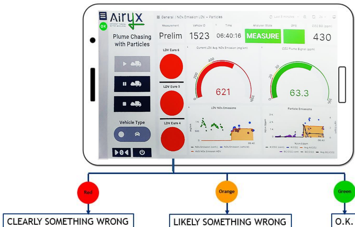
Figure 11: Explanation of the emission display as visualised during the measurement.
