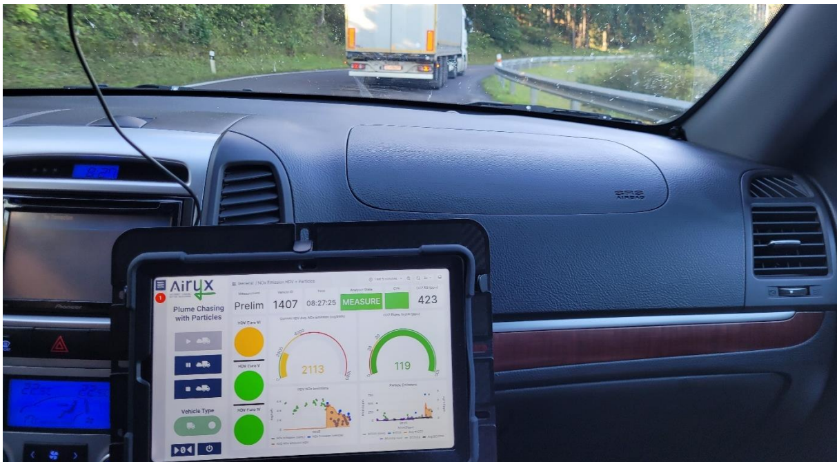
Figure 9: Display installation in the cockpit. A tablet is used to display the real time data and is connected via WiFi to the ICAD instrument. It allows operation and visualisation.
