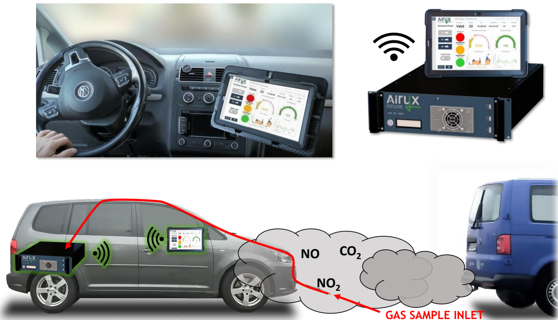
Figure 4: Basic sketch of plume chasing measurement principle from Airyx GmbH. The diluted exhaust gases are sampled and analysed. Different gases are measured with the ICAD-NO x -200DE instrument (NO 2 , NO x , CO 2 ) and particles are measured with (not shown in this illustration) Black Carbon Tracker (BC) from TUG and AVL DiTEST Counter (PN). From the ratio of the gases and particles, emission factors of the followed vehicle are derived.
